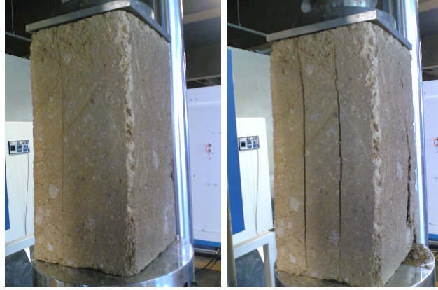
Fig. 5. Cracks during the uniaxial compression test in the parallel direction to the two layers. (a) Left: the first crack that appears fairly early on in the test is located between the second and the third (last) layer. (b) Right: the second crack that appears towards the end of the test is located between the first and the second layer.
